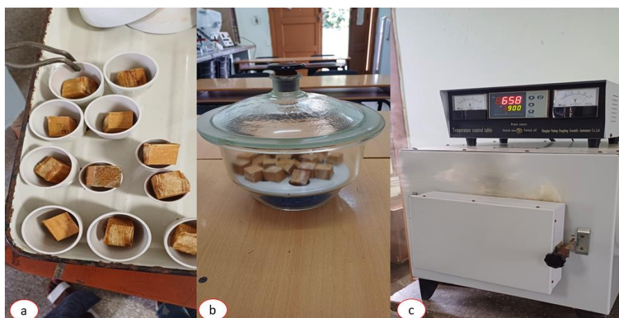
Figure 3. - Laboratory materials and equipment. a- crucibles, b- desiccator, c- muffle
