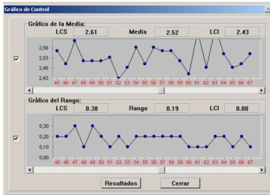
Fig. 3. - Graphic display of the sawing variation for pieces of 4 m length
