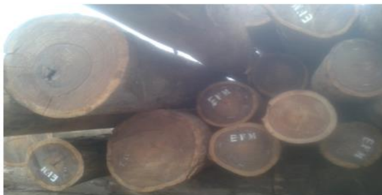
Figure 5 - Tiama logs with ovality
