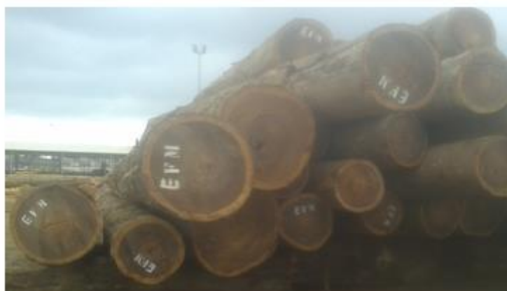
Figure 4 - Tiama logs with eccentricity
